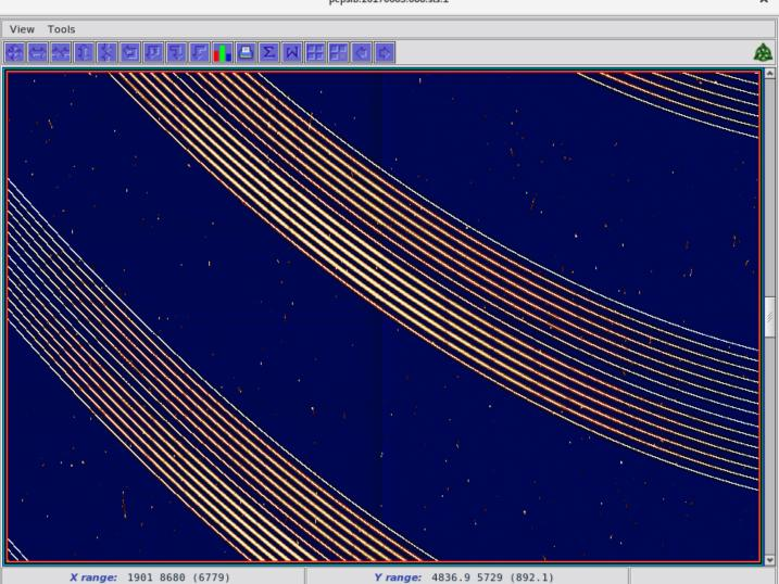
The order definition is obtained from the tracing flat field exposures made separately for each image slicer. The overall curvature and its sign is obtained from the global cross-correlation of all orders. The Gaussian profile elongated along polynomial path is matched to each slice of every order to form a 3D matrix of Chebyshev polynomials coefficients for the final global fit. Shown a fragment of the image with two image slicers and their traces.
