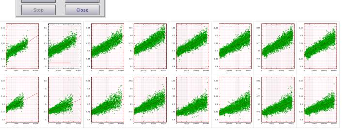
The STA1600 CCD gain calibration is done for each of its 16 amplifiers by using the ratio of two de-focused images of master flat field images repeated at different illumination levels. The conversion factor is the intercept of the fitted line to the gain factor as a function of ADUs. The variance for each pixel is estimated according to the linear fit.
