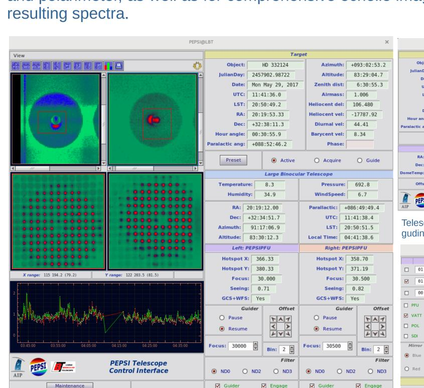
PFU IIF control interface with LBT for presetting to the target and keepeing it centered on the fiber pinhole during integration.
