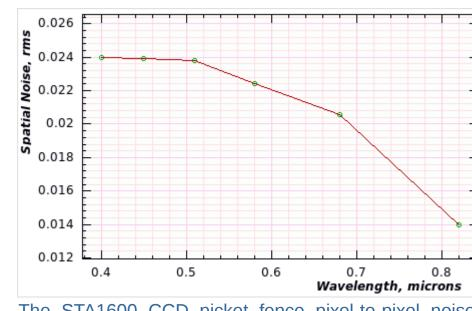
The STA1600 CCD picket fence pixel-to-pixel noise rms versus wavelength requires that the master flats are taken for each cross-disperser separately as the sum of hundreds of exposures. Furthermore, each pixel shows it own non-linear response to different illumination levels, therefore, a polynomial approximation is used to for a super-master flat versus illumination level in order to correct for the CCD spatial noise pattern for each pixel.
