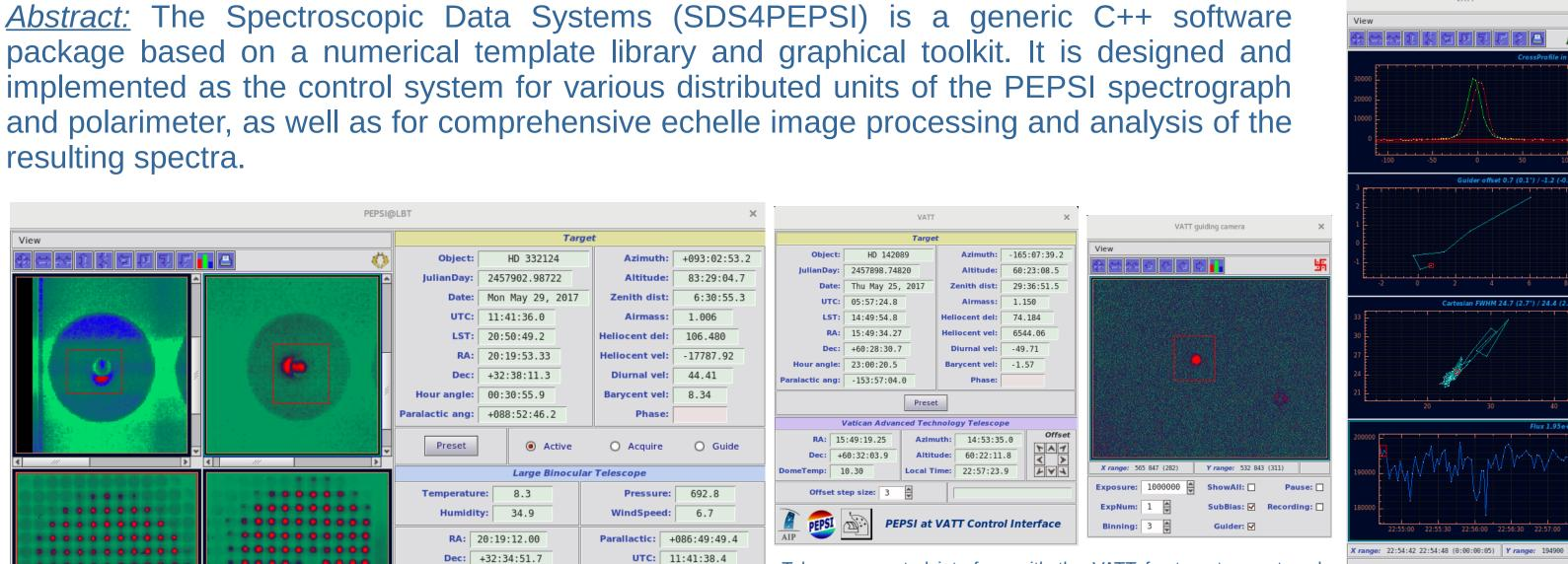
Telescope control interface with the VATT for target preset and guding on the direct-reflected image during integration.
