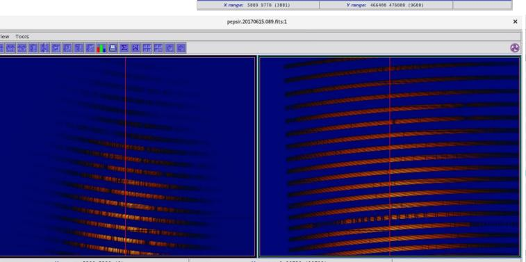
The image and spectrum viewer allows to measure the signal/noise of the exposed images at the selected region of interest. The table shows the selected parameters from the image FITS headers after each new image is added after last exposure.
