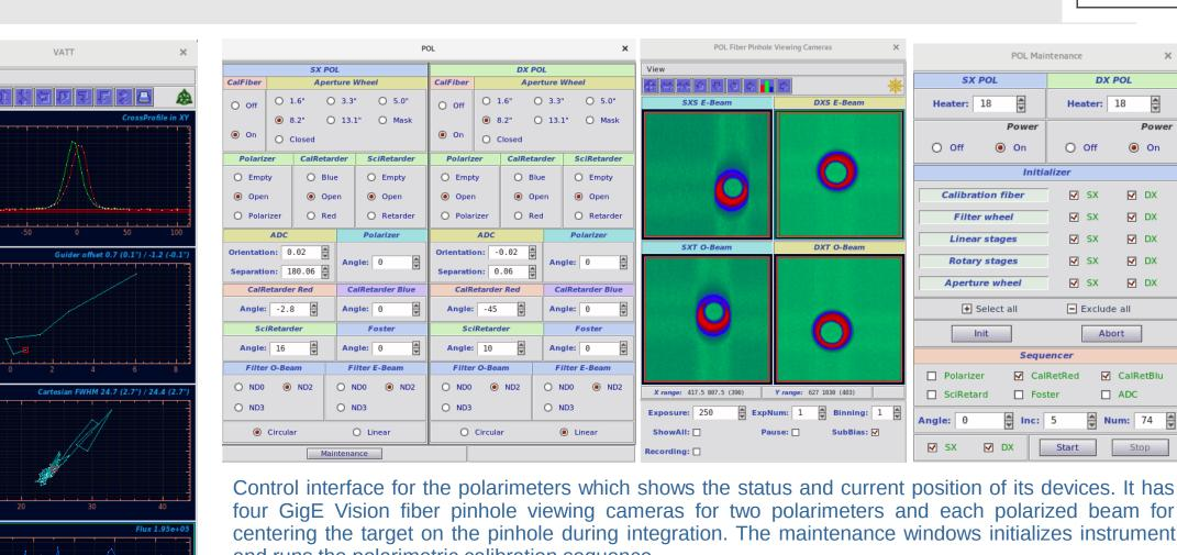
four GigE Vision fiber pinhole viewing cameras for two polarimeters and each polarized beam for centering the target on the pinhole during integration. The maintenance windows initializes instrument and runs the polarimetric calibration sequence.
