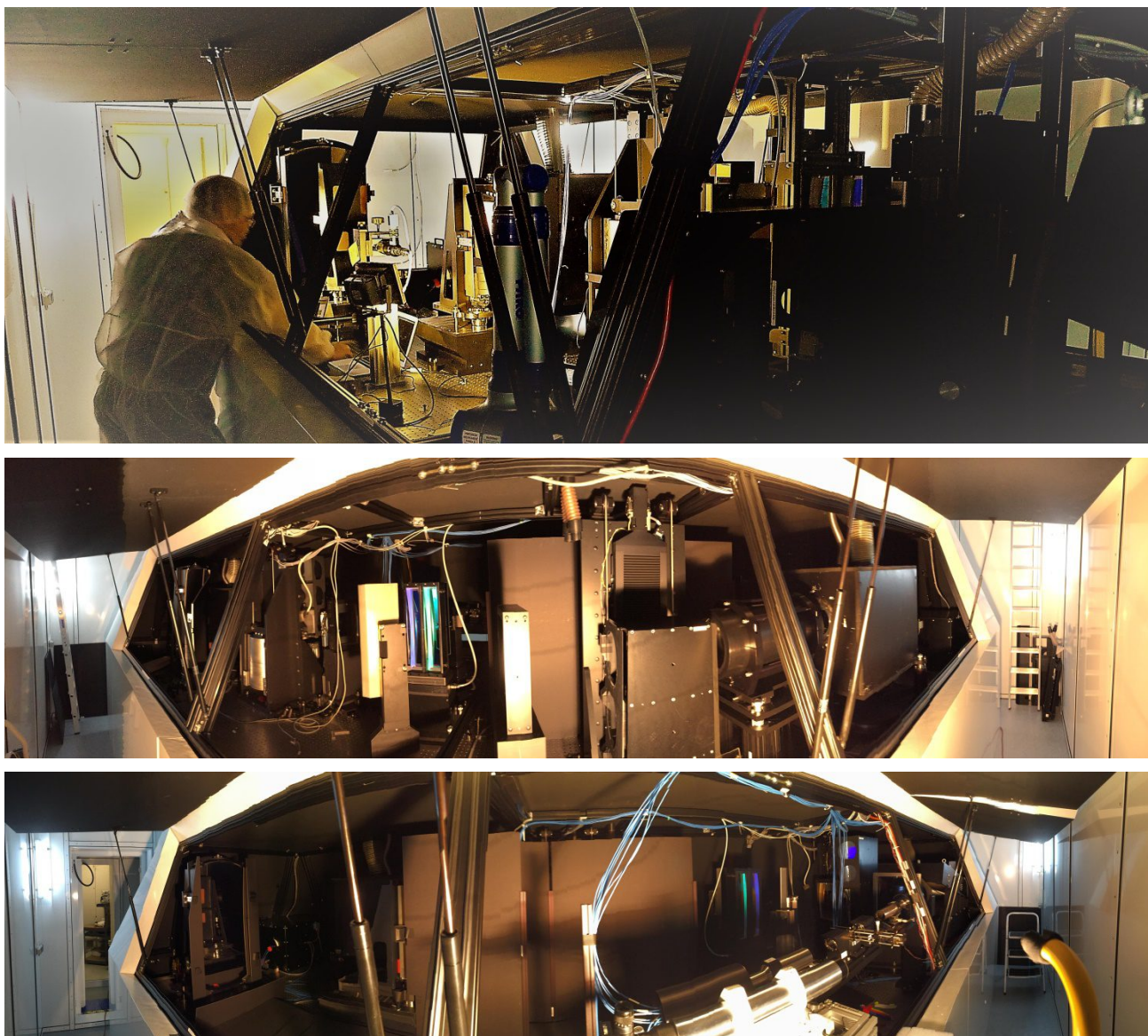
Figure 2. Open hatches of the inner cover around the spectrograph. The table dimensions are 6×2m. Top : On the left edge is the main collimator mirror seen, the blue-arm transfer collimator mirror is just close-by to the right. The grating is in the black box to the very right of the picture. Middle : panoramic view of the red-arm side. Bottom : panoramic view of the blue side-arm side.
