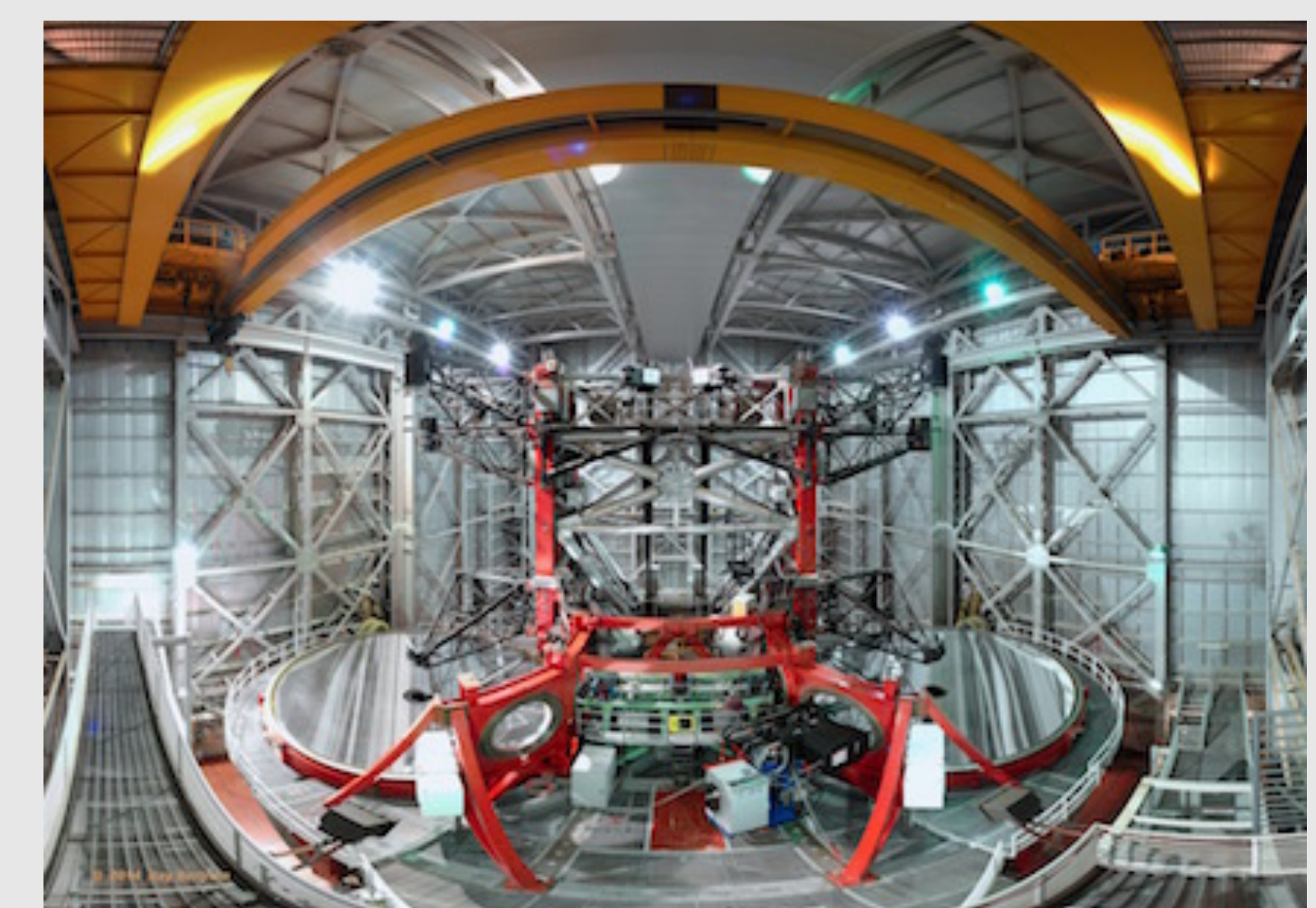
2 \times 8.4 m Large Binocular Telescope with the PEPSI Permanent Focal Units (large white boxes mounted to the structure bottom and left and right of center).
